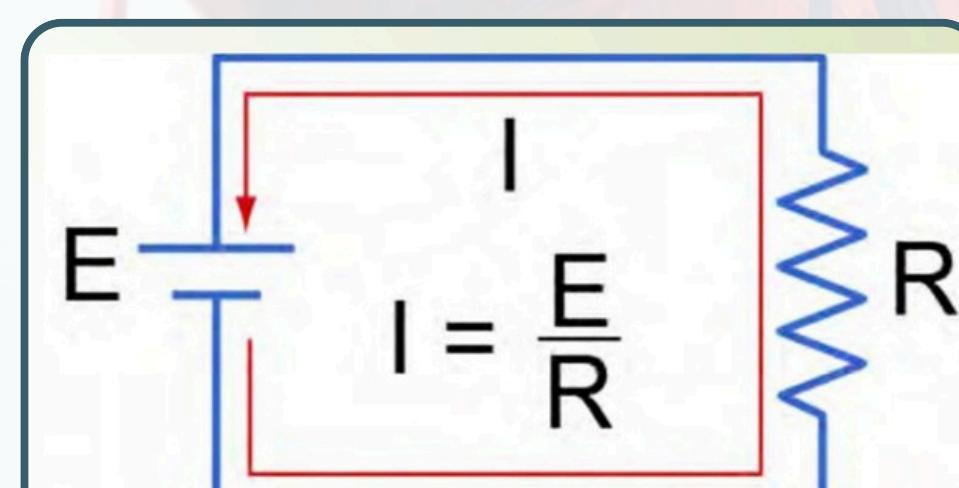
Current (I) is measured in amperes (amps)
