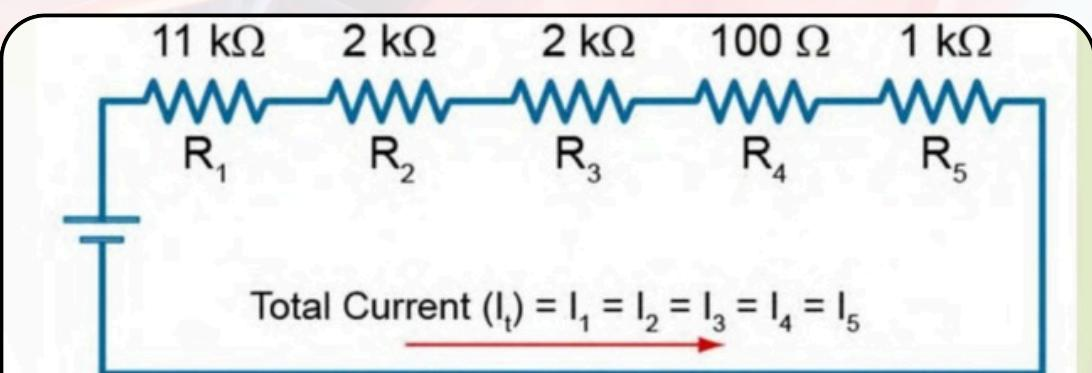
$$\text{Total Resistance} = R_t = R_1 + R_2 + R_3 + R_4 + R_5$$
